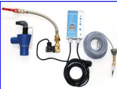
**Mains Water Top Up Set.** The Level Probe senses tank water level. At low water level the solenoid valve opens. The Control Unit switches a connected pump (not included) on and off, to save it from running dry. The Control Unit prevents the solenoid valve blocking, by testing it periodically (3 per wk).
